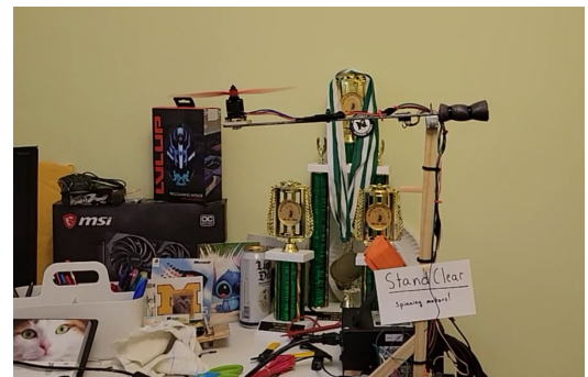
Running a single tethered rotor on my “PID test” jig
